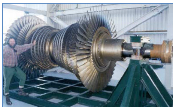
Figure 4: View of the rotor equipping one of the units of the power station in Larderello in Italy (©Geo-heatcenter).
