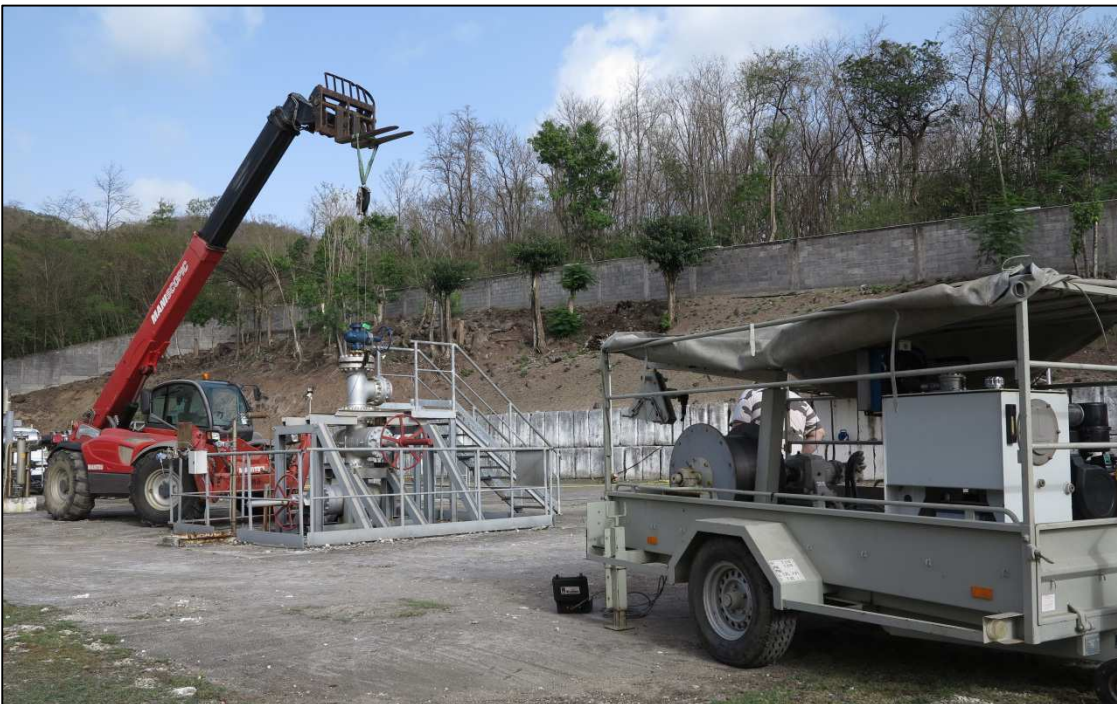
Figure 1: Used equipment during the measure of the pressure and the temperature in a geothermic well in the field Bouillant in Guadeloupe.
